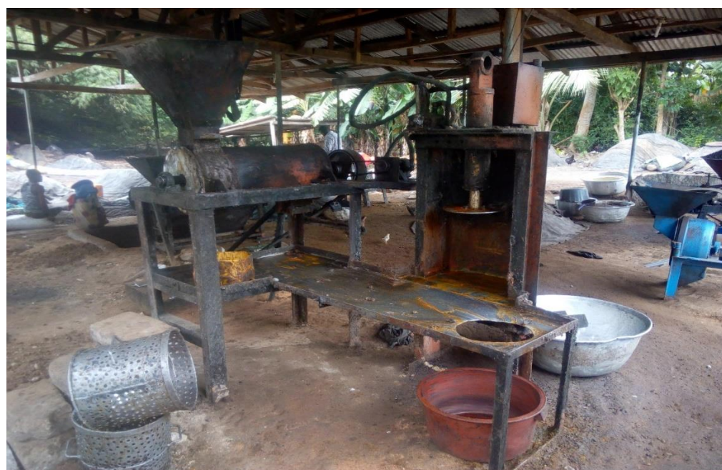
Figure 8: Hydraulic press machine (Brofoyedru Co-operative)
