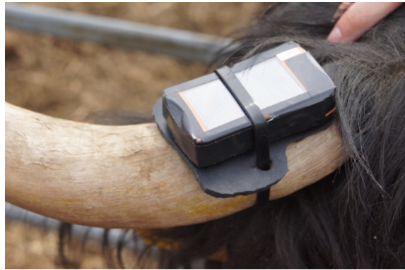
Figure 9: GPS attachment to the base of the horn
