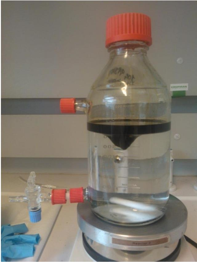
Figure 1 glass aspirator flask connected with glass tube and closed off with rotary switch
