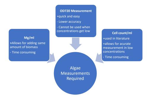
Figure 7: The pros and cons of the different typed of algae measurements required for this research.
