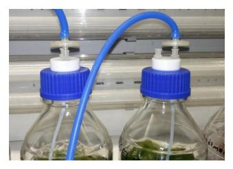
Figure 2: culture vessel with air filter and input / output cap
