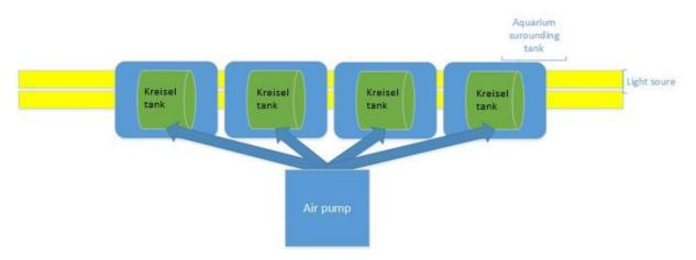
Figure 9: experimental setup larvae tests: pressurized air is pumped to aerate four Kreisel tanks submerged in aquaria.
