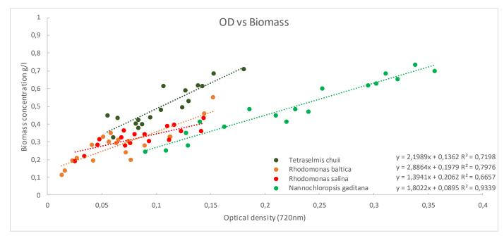
Figure 12: Optical density (720nm) on the X axis correlated with gram per litre on the Y axis for Tetraselmis chuii, Rhodomonas baltica, Rhodomonas salina and Nannochloropsis gaditana
