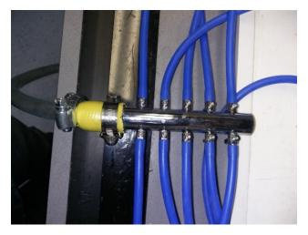
Figure 1: air being split to different culture vessels
