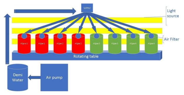
Figure 5: Schematic overview algae growth setup. Pressurised air is first hydrated through demi water and then divided over the 8 bottles, first passing an air filter of 0.2µm to minimize the risk of contamination.
