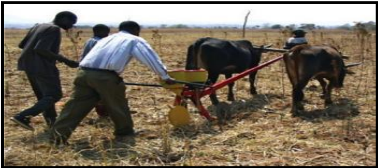
Figure 5: Direct seeder mounted on oxen. Source (Feed for the future, 2012).
