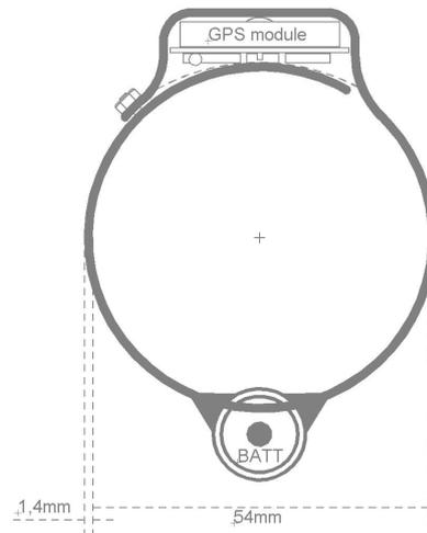
Figure 2. Cross section of a neck-collar with GPS-module built in (van Gils).
