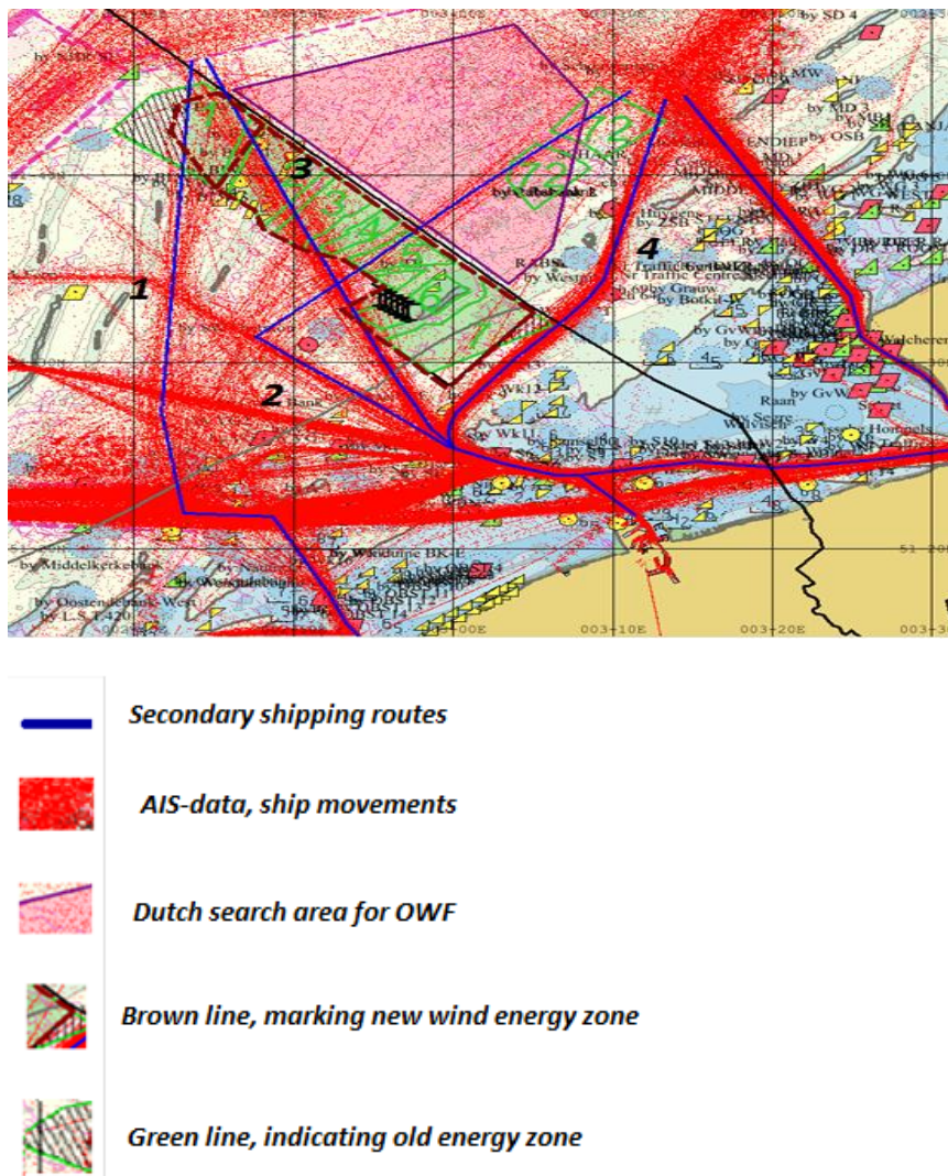
Figure 5, The numbers 1-4 are showing the routes which will be partly or fully cut off by the construction of the wind farms in the concession zone. The red lines indicate the ship movements during one month. The blue lines indicate the secondary shipping routes which will be cut off (A.Michaux 2009-2010).
