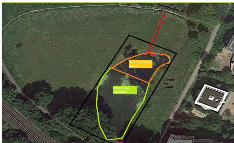
Figure 11: The retention basin with possible application of sedimentation and infiltration structure (Google maps, 2014).
