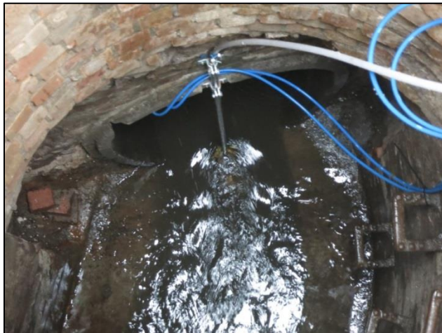
Figure 20: Litter trapped on steel pipe and sampling tube, causing rinse errors and missed samples.
