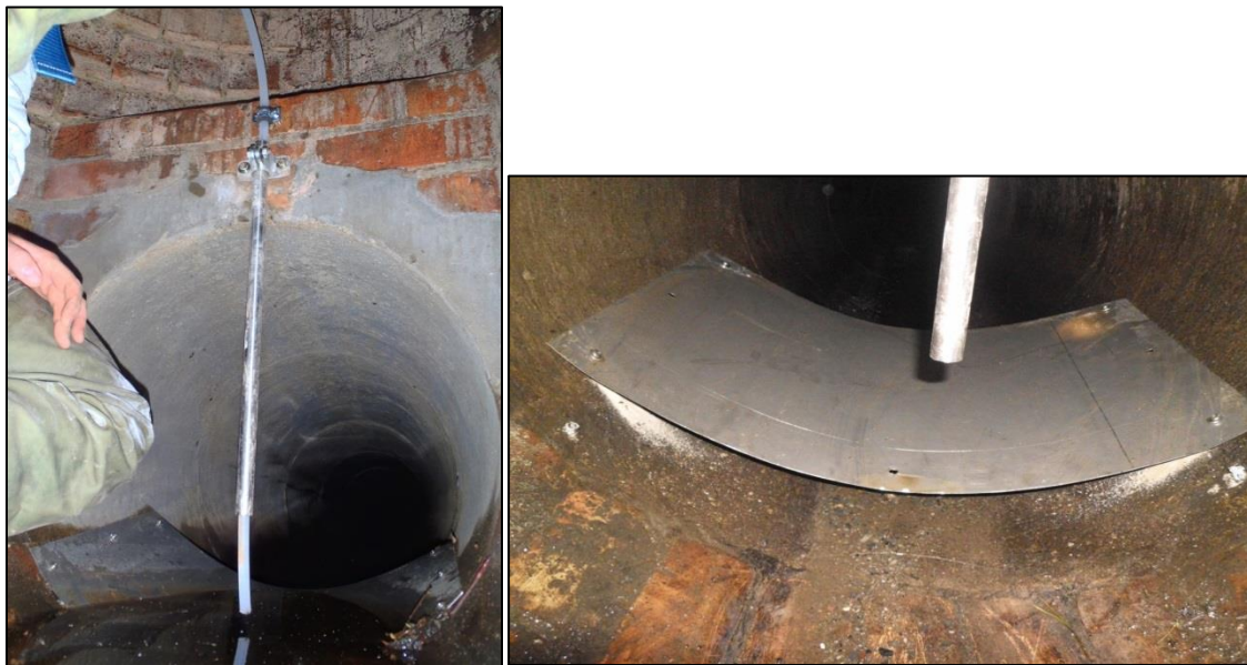
Figure 26: Steel pipe, sampler tube and steel plate after initial installation (left) and after modification (right).
