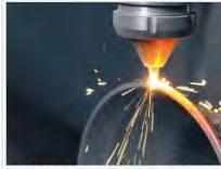
Laser deposition welding by DMG Mori
