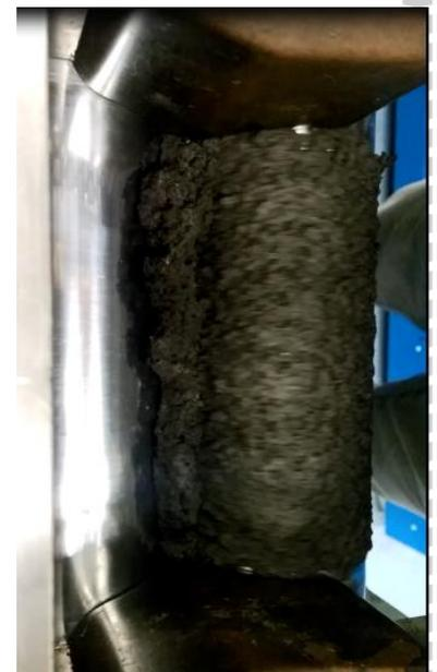
Figure 11, Milling of devulcanized rubber
