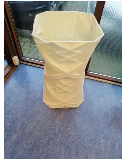
Figure 20 3D printed trashcan made of FRP's
