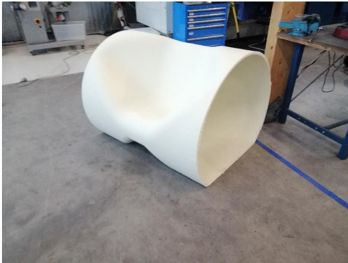
Figure 19 3D printed bench made of FRP's
