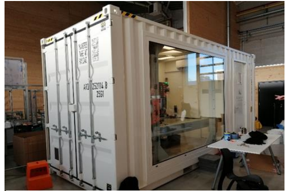
Figure 6 Colossus 3D Printer
