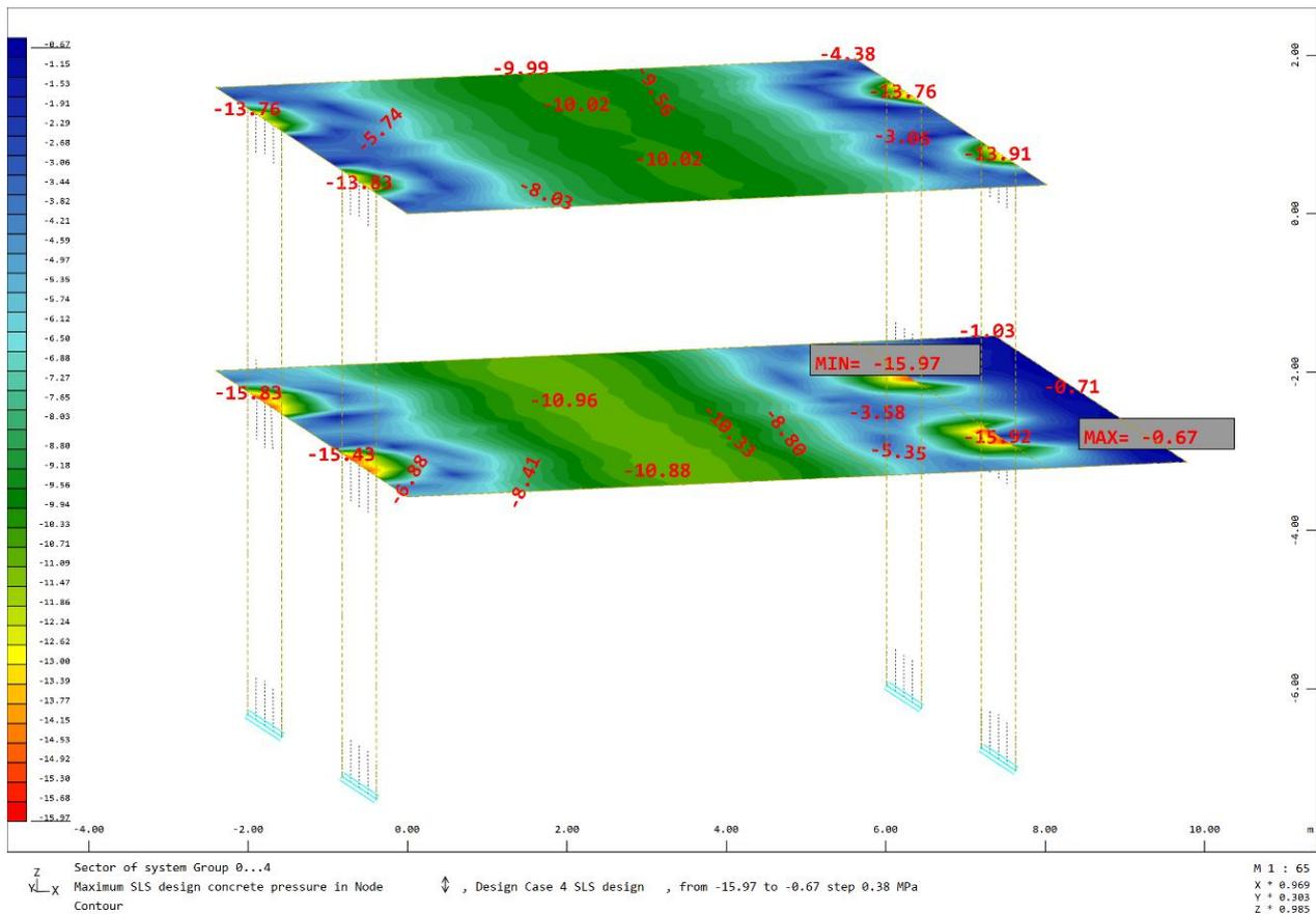
Figure 48: Compressive Stresses in rare SLS
