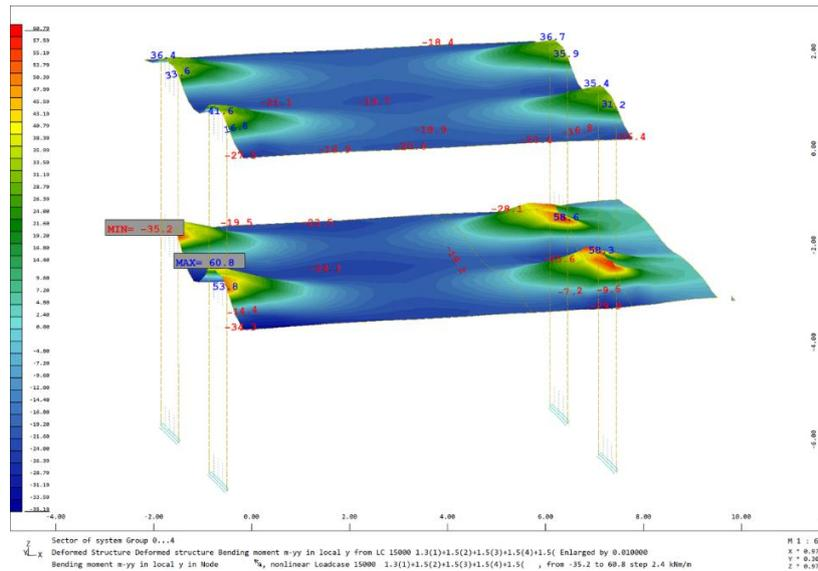
Figure 40: Bending moments along y direction
