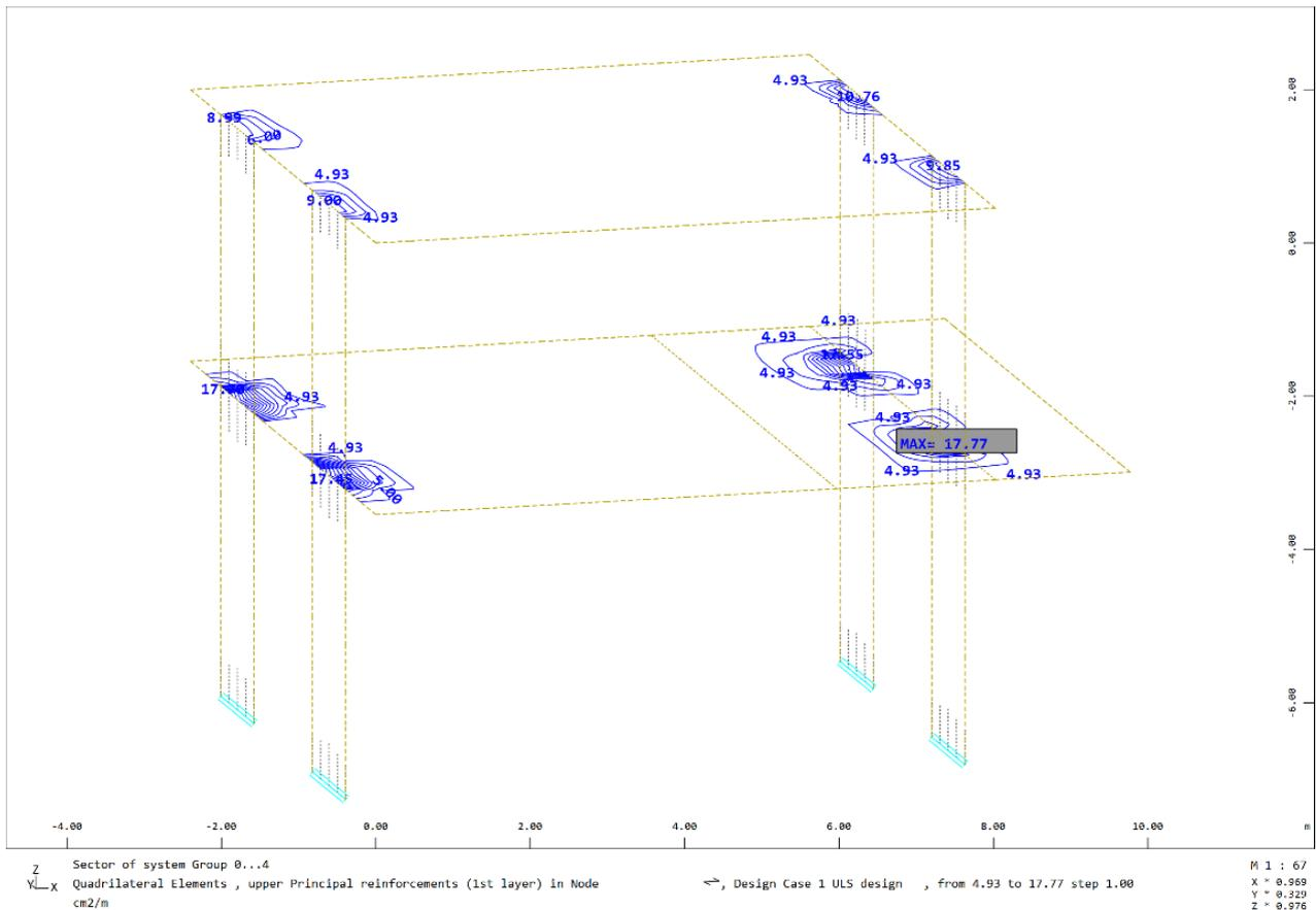
Figure 43: Upper Principal Reinforcement
