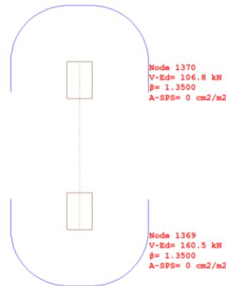
Figure 89: Punching Shear Check for bearing walls
