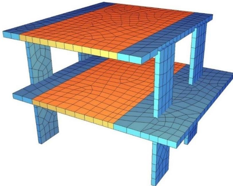
Figure 77: finite element model - Alternative 3
