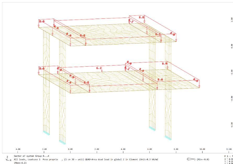
Figure 72: Self-weight of slabs - Alternative 2
