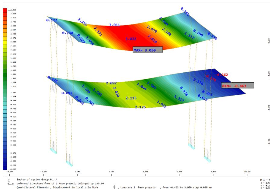
Figure 73: Deformations - Alternative 2
