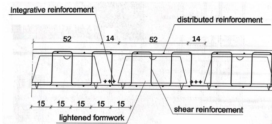
Figure 54: Positioning of shear reinforcement
