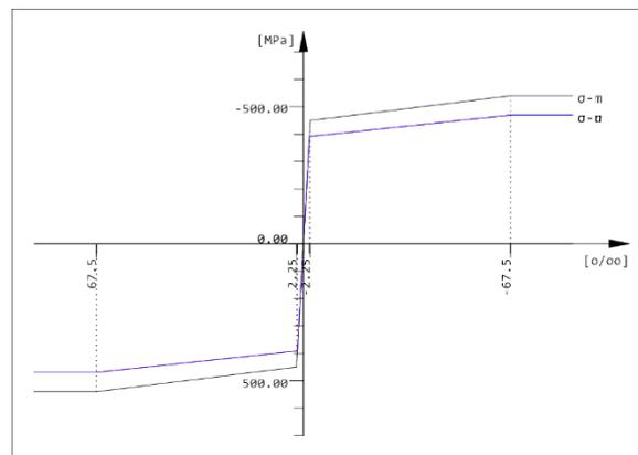
Figure 25: Stress-strain curve - B 450 C
