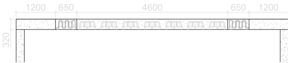
Figure 59: Longitudinal cross-section - Roof slab
