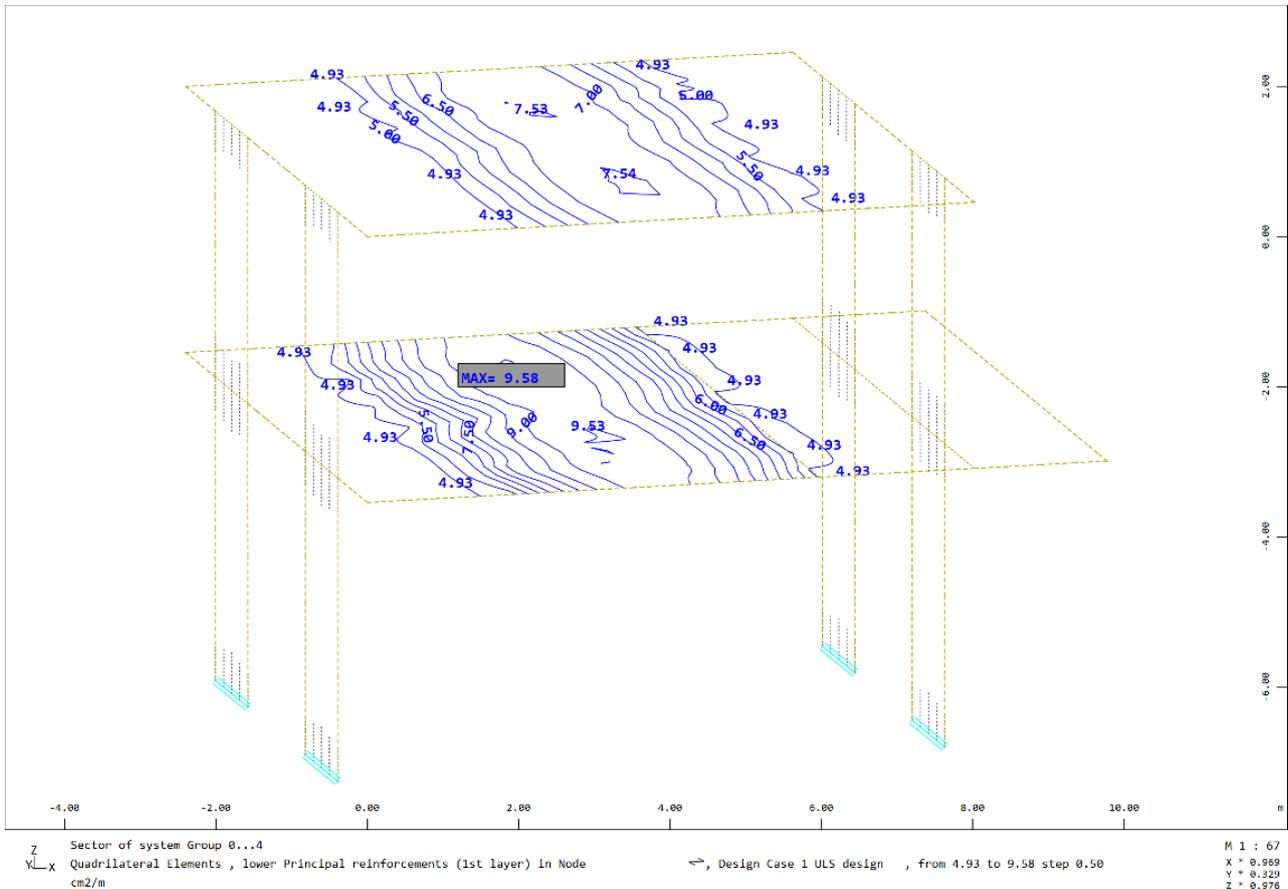
Figure 44: Lower principal reinforcement
