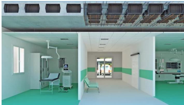
Figure 62: Voided slab section
