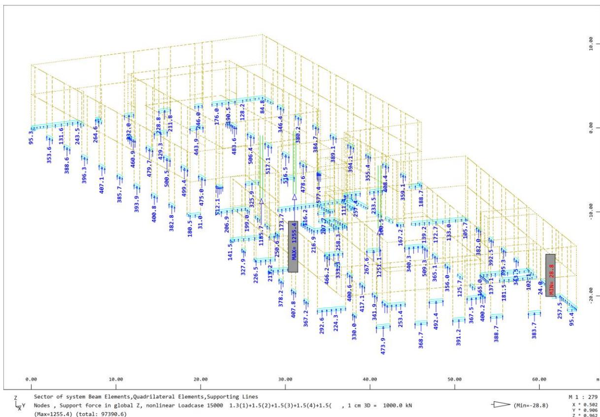
Figure 94: Support reactions - standard model
