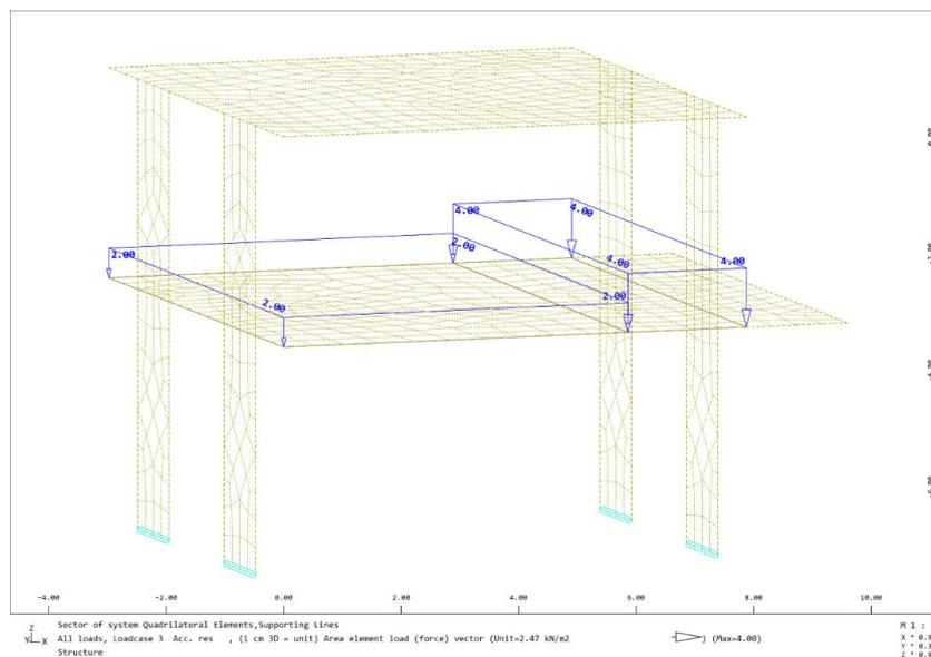
Figure 34: Variable loads on the intern
