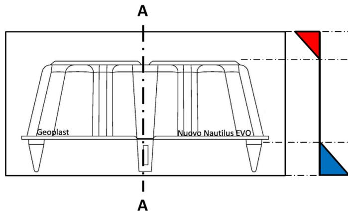
Figure 68: Expected stress-diagram in lightened slab section
