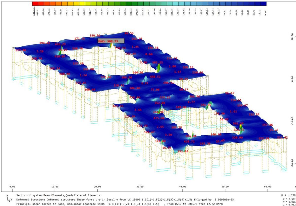
Figure 91: Shear Forces - Roof Slab
