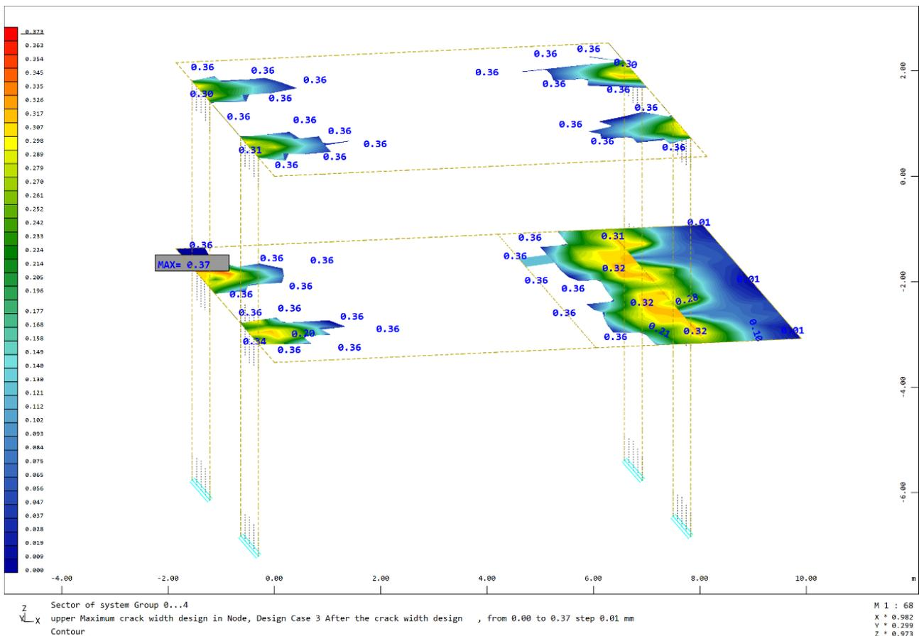
Figure 46: Expected cracks in frequent SLS
