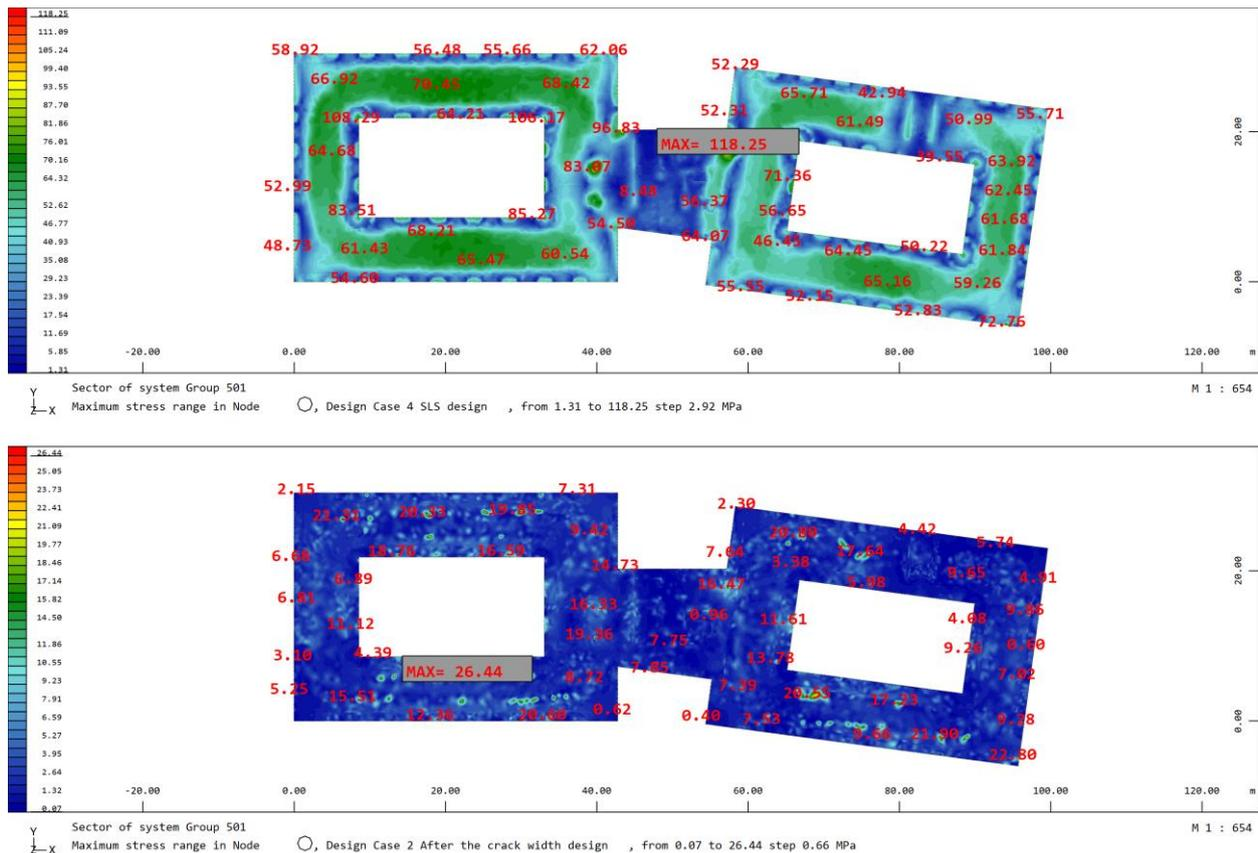
Figure 106: Steel tensions in Roof slab
