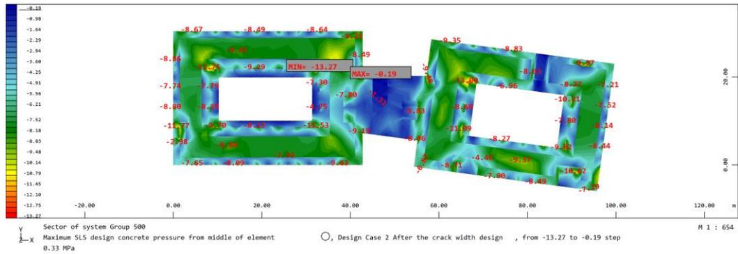
Figure 103: Concrete tension - first-floor slab
