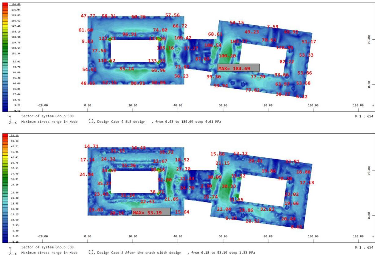
Figure 105: Steel tensions in first-floor slab
