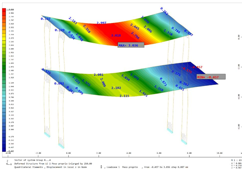
Figure 66: Deformations - Alternative 1
