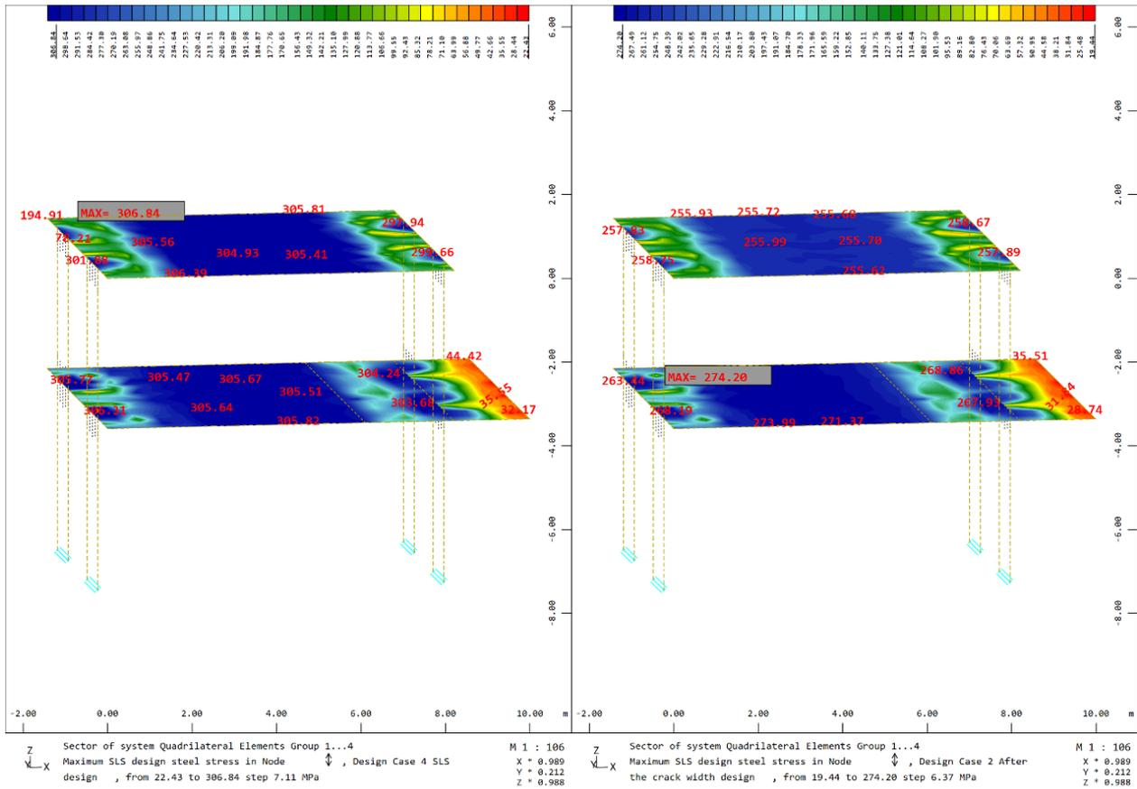
Figure 50: Steel Tensions
