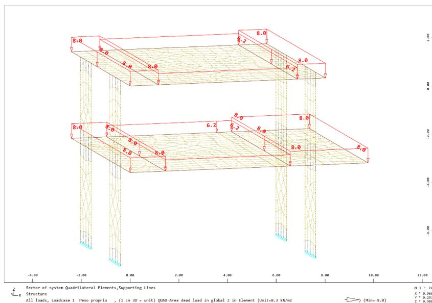
Figure 65: Self-weight of slabs - Alternative 1
