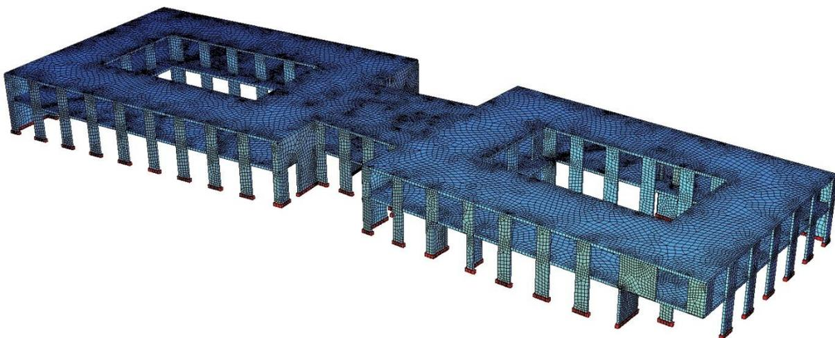
Figure 84: FEM Model of Casa Haus inge - view 2
