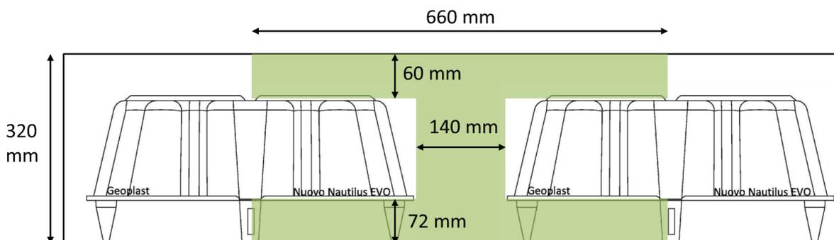
Figure 52: H-section of reinforced concrete
