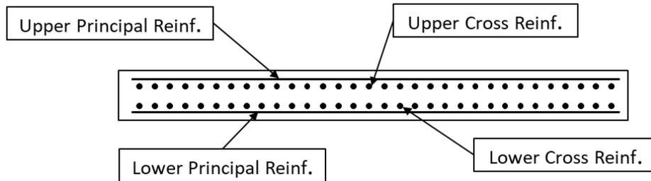
Figure 42: Cross-sectional view of generic slab
