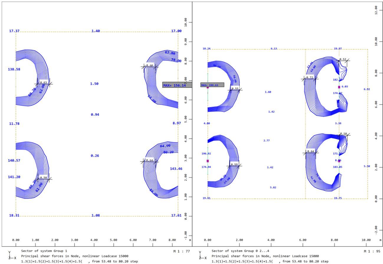
Figure 57: Lightened section with shear reinforcement
