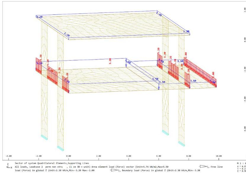
Figure 33: Permanent non-structural loads
