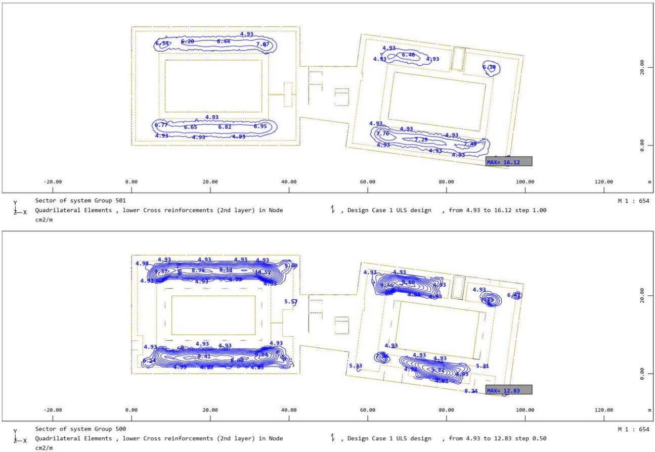
Figure 99: lower cross reinforcement
