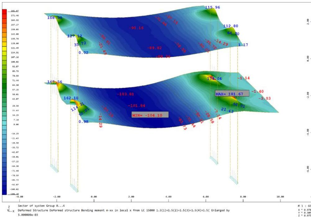
Figure 39: Bending moments along x direction
