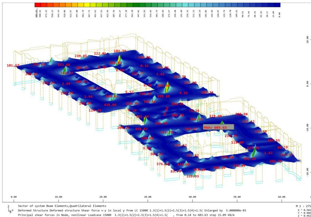
Figure 90: Shear Forces - First-floor slab
