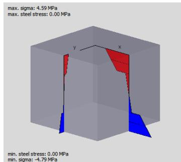
Figure 81: Concrete's stress-diagram
