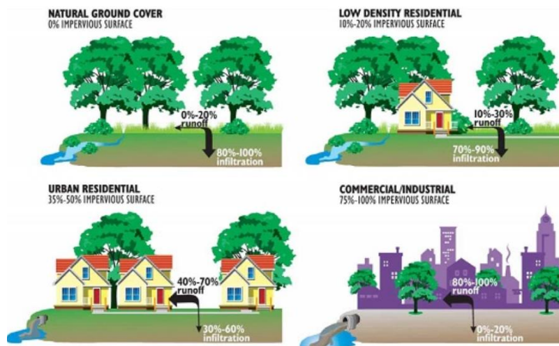
Figure 4: Changes in hydrology and runoff due to urbanization (Juneau Watershed Partnership, 2018).
