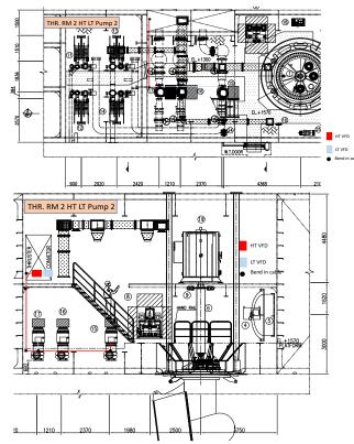
Figure 33 Thruster room 2 wiring plan (L.J.M. Verboven, 2023)
