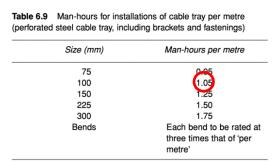
Figure 9 Man-hours for installations of cable tray per metre (Butler, 2012).
