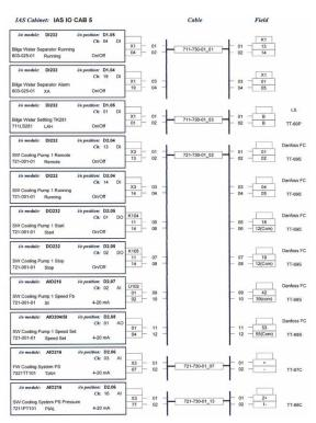
Figure 18 example of a IAS IO Cabinet with channels reserved for VFD
