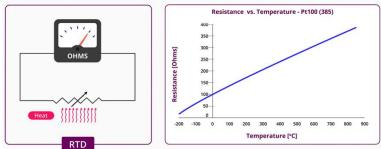
Figure 8 Block diagram of a RTD and the linear relation between temperature and resistance of the PT-100 (Sommer, 2022)
