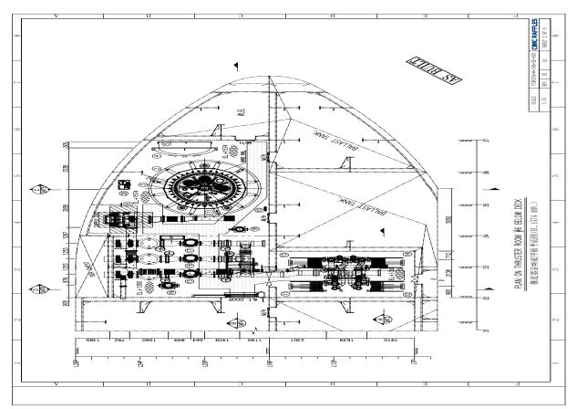
Figure 24 Top view of Thruster Room #6 Source OOS International (2022).
