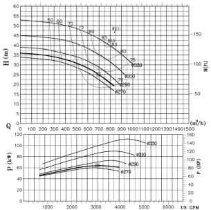
Figure 13 Pump curve and absorbed power of HT LT SW cooling pump (Azcue pump manual).
