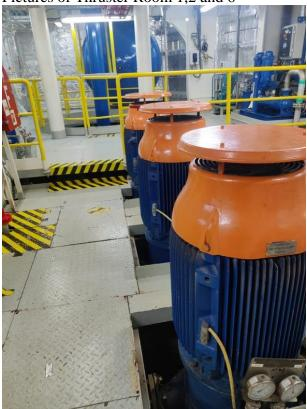
Figure 25 Thruster Room 1 LT HT pump 3 (Starboard side pontoon). Source L.J.M. Verboven (2022)
