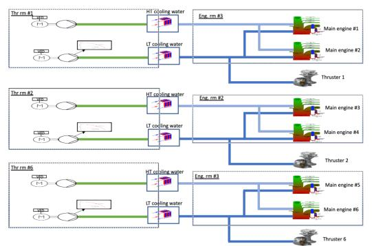
Figure 1 Overview of the six cooling pumps that will be discussed in this research. The idea is to upgrade the motors with variable frequency drives (VFD'S) as seen in the figure. (L.J.M. Verboven, 2023)
