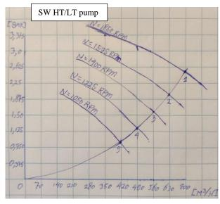
*Figure 14 Pump curve for seawater HT/LT pump (L.J.M. Verboven, 2022).*
