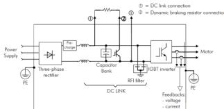
Figure 4 Block diagram of variable frequency drive
