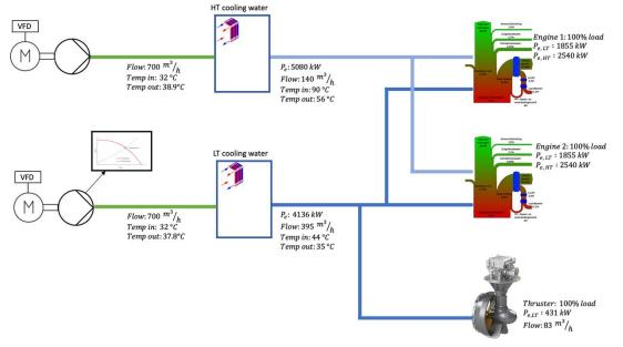
Figure 12 Simplified overview of SW for supply vs Demand on FW system at 100% load (L.J.M. Verboven, 2023).
