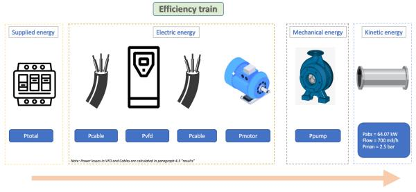
Figure 15 Efficiency train (L.J.M. Verboven, 2023).
