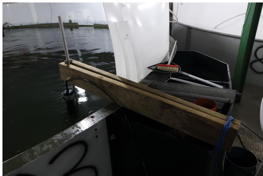
Figure 3.8: Acoustic velocity measurements in commercial scale tanks in Lensvik.
