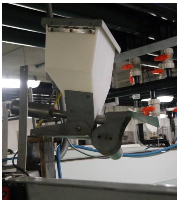
Figure 3.5: Feeding machine attached to the side of a 3,2 m 3 rearing unit at the Nofima centre for recirculation.
