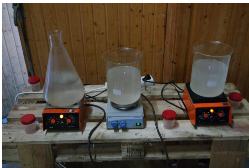
Figure 3.12: Preparation of stock solution. Feed pellets were dissolved during 24 hours using a magnetic stirrer.
