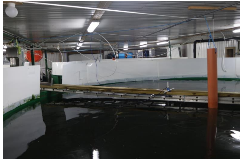
Figure 3.9: A ladder being used in order to create a tank profile displaying water velocities in commercial scale rearing units at Lensvik.
