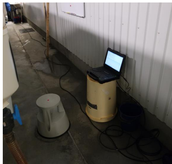
Figure 5.1: Computer attached to the Vector instrument during measurements running the accompanying software. This computer was used to operate the instrument and monitor the measurements.
