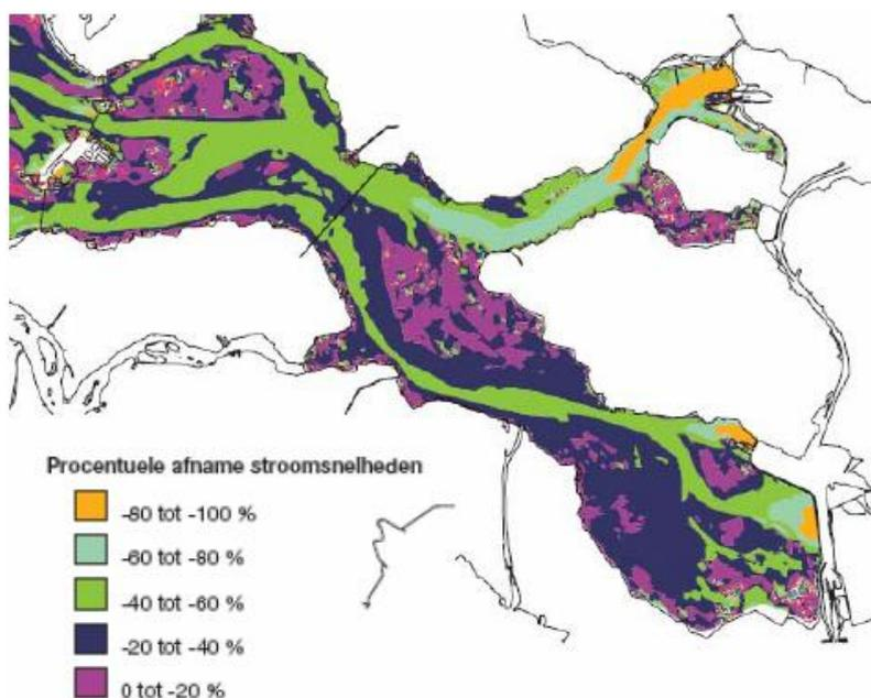
Figure 1.2.2 Decrease in flow velocities in the Eastern Scheldt after the construction of the storm surge barrier (Hoeven, 2006)
