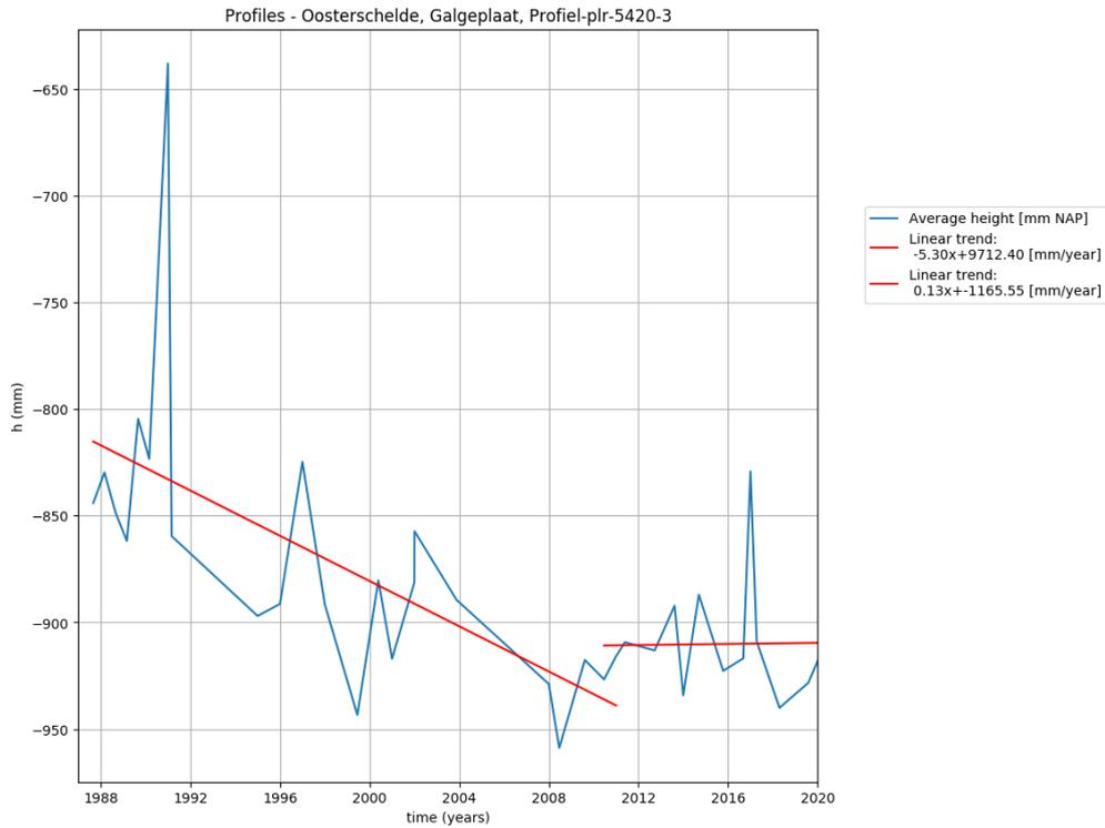
Figure 4.3.4 Profile 5420 and the trendline of the height (Rijkswaterstaat) with a breakpoint
