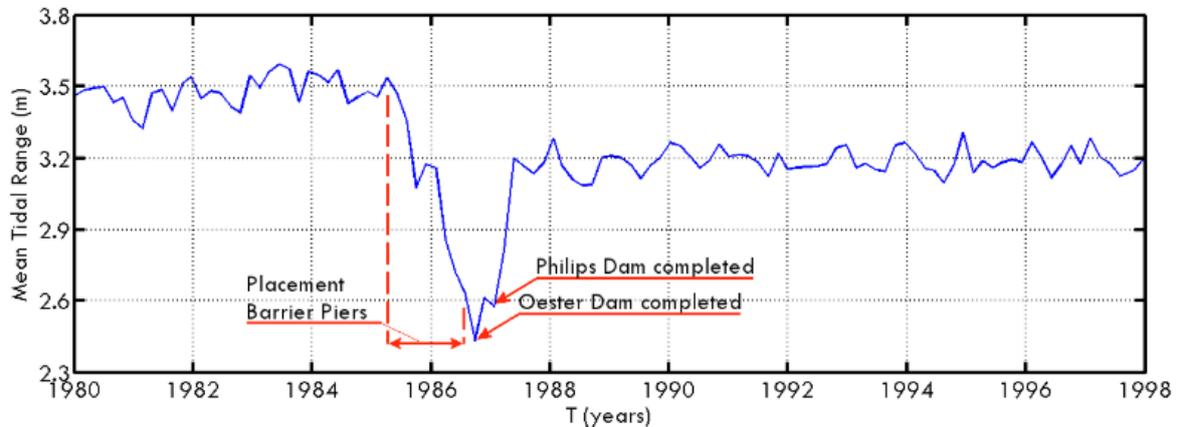
Figure 1.2.1 Changes in the mean tidal range of the Eastern Scheldt from 1980 to 1998 due to the Delta Project (Mulder, 1994)
