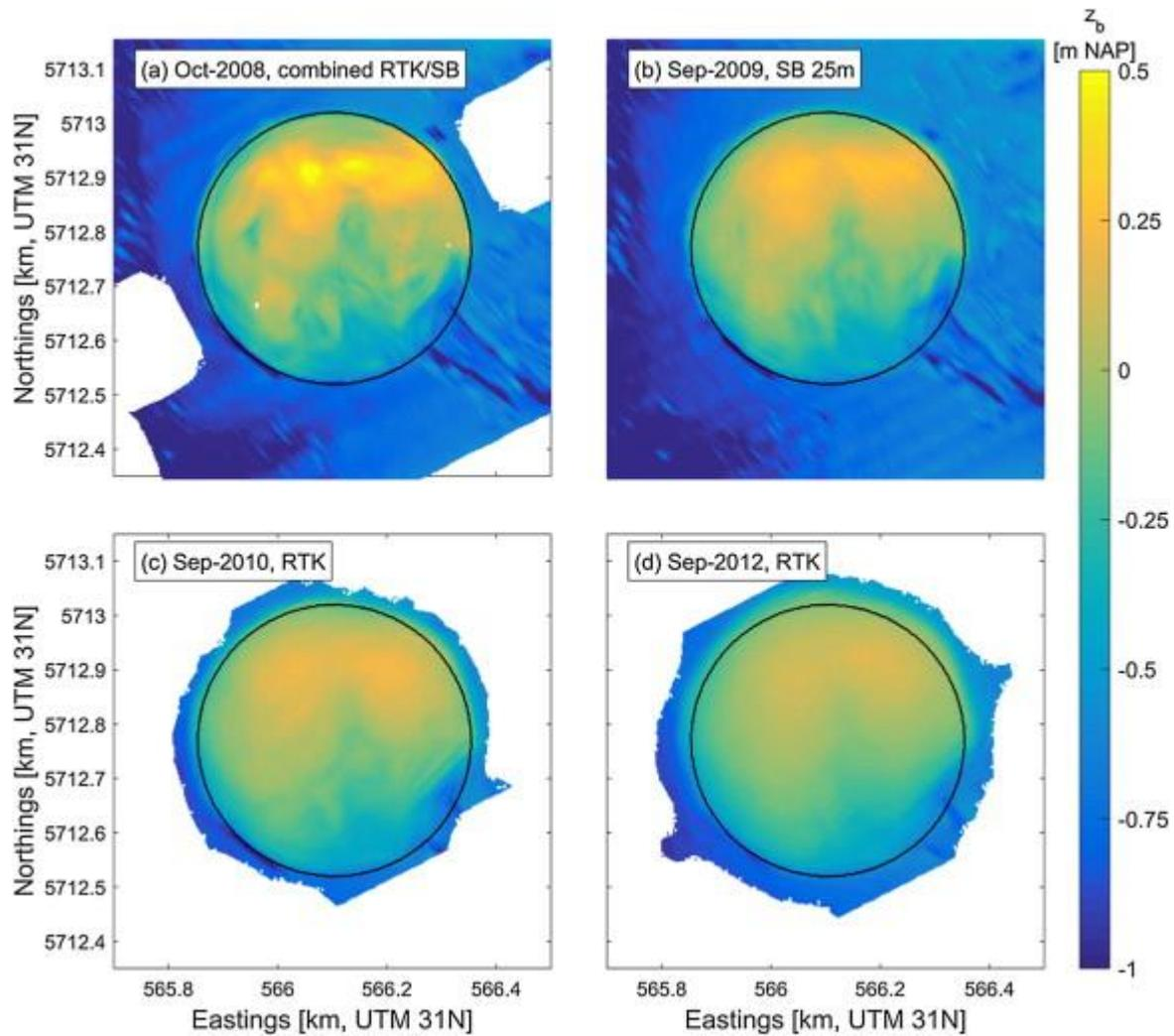
Figure 2.1.1 The changes in the bed level over four years after the pilot nourishment on the Galgeplaat (J. van der Werf et al., 2015).
