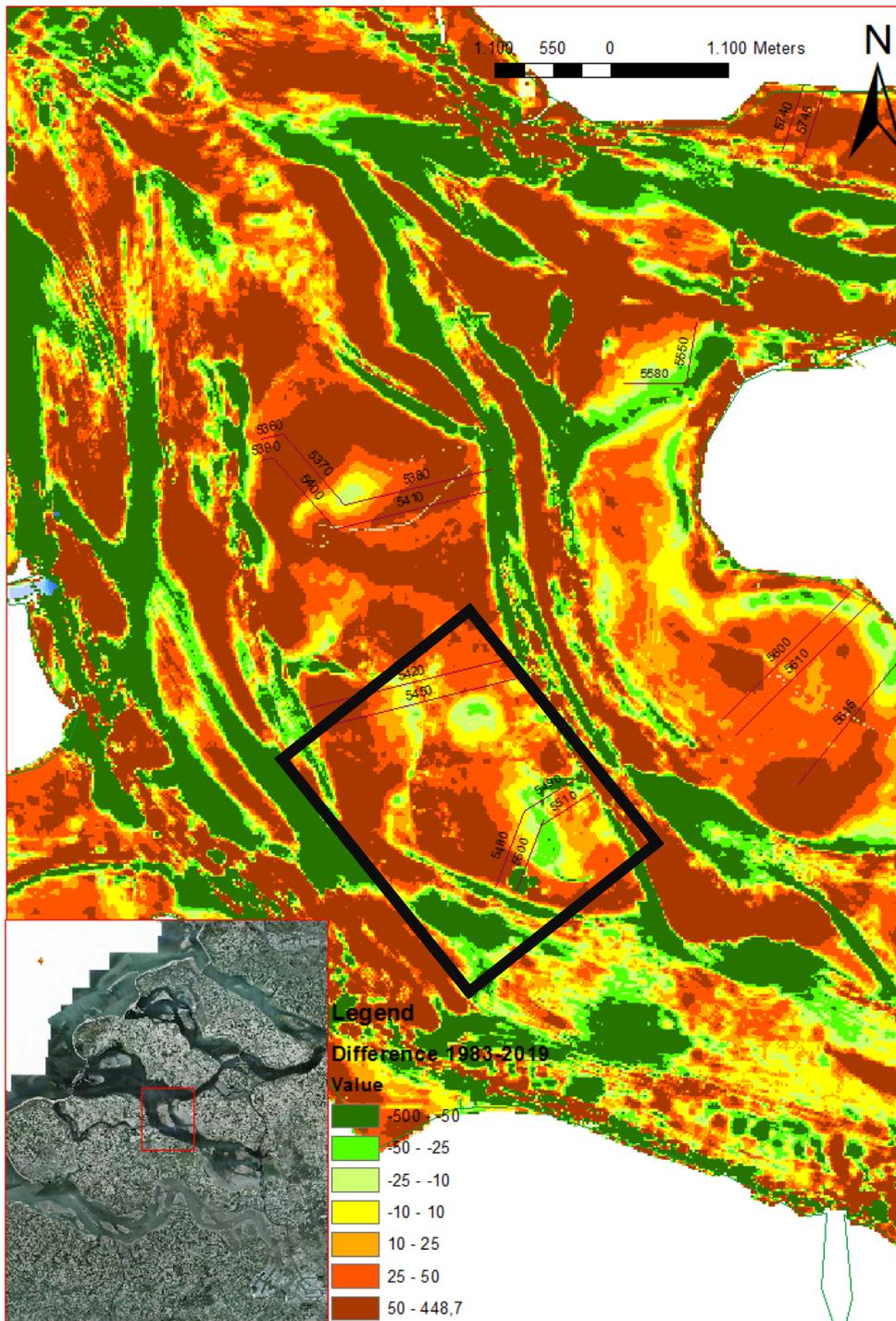
Figure 4.2.2 Difference in cm in height on the Galgeplaat from 1983-2019 (Red colour is erosion and green colour is sedimentation)
