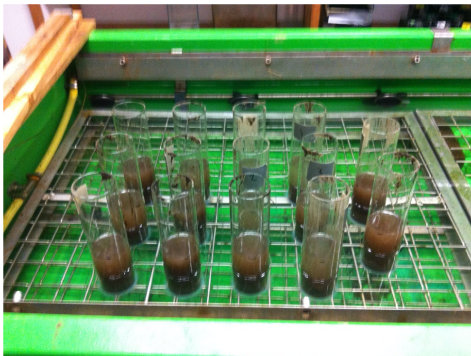
Figure 5: Experimental setup of the sugar pilot. Treatments consist out of duplicates which were randomly placed in a water bath
