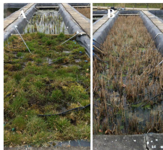
Figure 3: Biocascade (A) and helophyte filter (B) test ditches at the Radboud University
