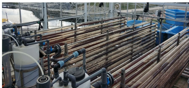
Fig. 1 Tubular photobioreactors located in Vlissingen and operated with R. salina
