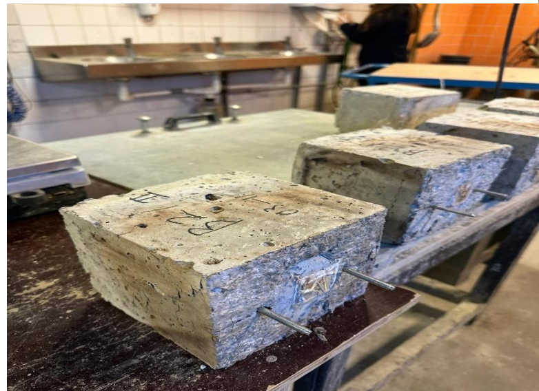
Figure 27: B2p Compressed After Fire
