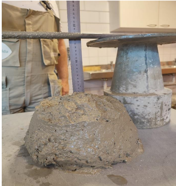
Figure 7: Slump Test of MixB1p - 16cm
