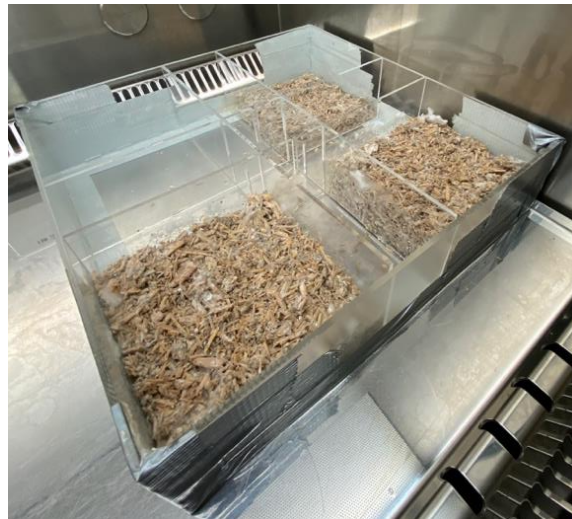
Figure 16: Mycelium in the molds ready for inoculation
