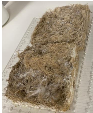
Figure 17: Mycelium composites after drying
