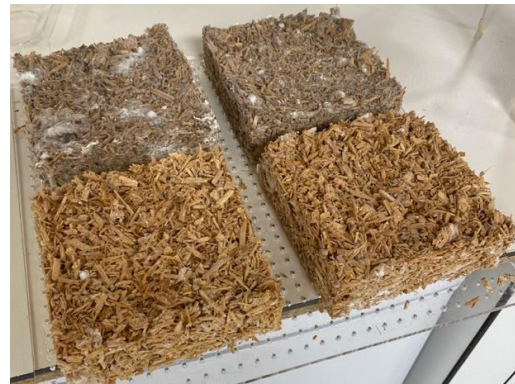
Figure 18: Mycelium composites after drying
