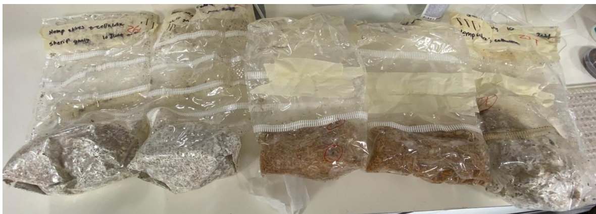
Figure 14: Mycelium bags after inoculation for 7 days
