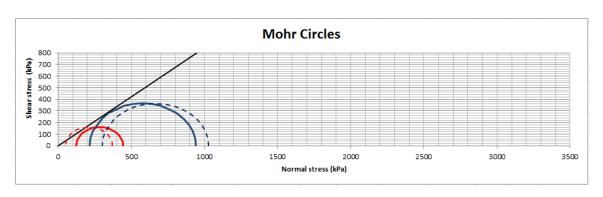
Figure 31 Mohr-Coulomb envelope for CU triaxial test at 7m depth
