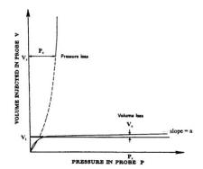
Note 1-The schematic graphs are not to scale; each calibration requires different volumes and pressures.
