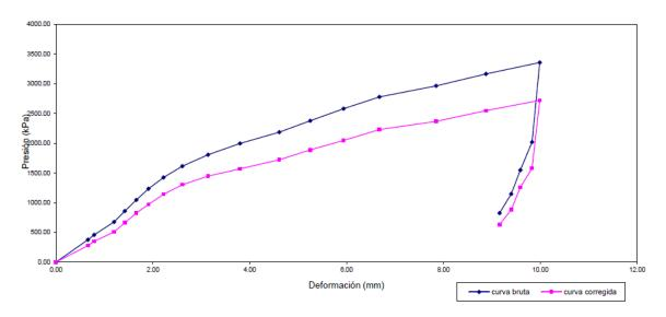
Figure 28 Actual and corrected curves of the pressure-volume relation at depth 7-7.5 m
