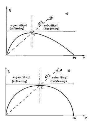
Figure 13 (a) Yield surface for cam clay model; (b) Yield surface for modified cam-clay model. (Potts & Gens, 1988)
