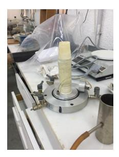
**Figure 17 Triaxial Test equipment**
