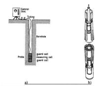
FIG. 1 a) Basic Principles of the Triple Cell Design Pressuremeter (Baguelin, Jézéquel and Shields, 1978,<sup>3</sup> b) Slotted Tube with Probe
