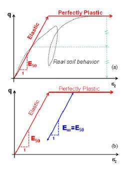
Figure 10 Elastic-perfectly and Plastic-perfectly assumption of MC model (Gouw, 2014)
