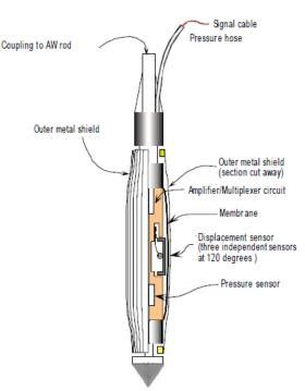
Figure 6 Schematic detail of the Pressuremeter. Source: (HOLT Engineering, 2009)
