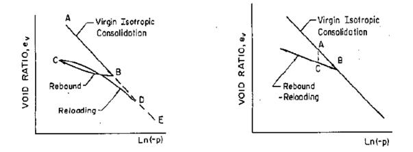
Figure 14 Response of real soil to hydrostatic stress and Response of idealized soil to hydrostatic stress. (Ti, 2009)
