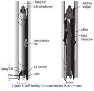
The Self-boring method is suitable for soils ranges from loose sand and soft clay to weak rock. Other materials, such as gravel and hard rock are not measured with self-boring instrument since it may damage the cutting edge. The self-boring technique usually takes part in 60 meters depth or more for a vertical hole. It also required the modest amount of reaction and less supporting tools, especially for soft clay.
