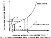
FIG. 8 Pressuremeter Test Curves for Procedure A
