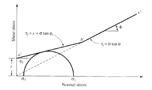
Figure 18 Typical Total stress failure from CU test in OC clay
