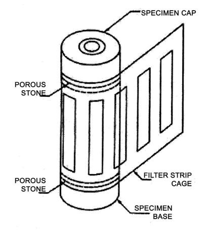
FIG. 2 Filter Strip Cage
