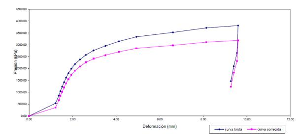
Figure 29 Actual and corrected curves of the pressure-volume relation at depth 9-9.5 m
