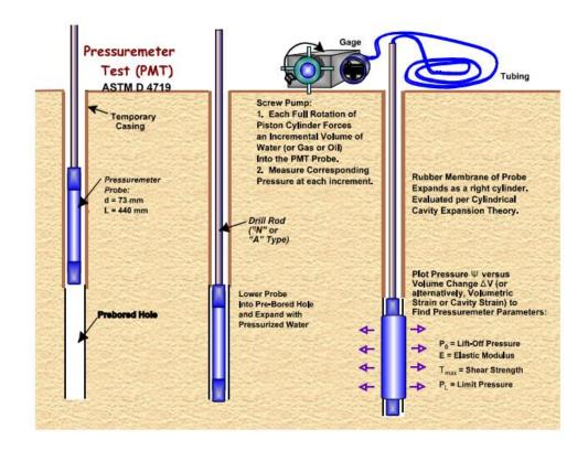
Figure 7 Procedures of Pre-bored Pressuremeter test (GeotechnicalDesign.Info, 2017)
