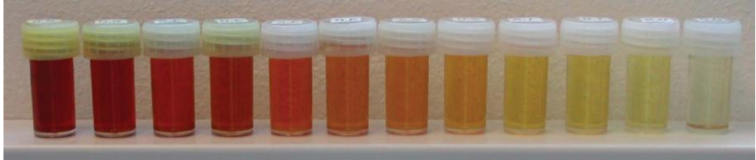
Figure 2-3: Example oil colours for a regeneration (Source ABB)
